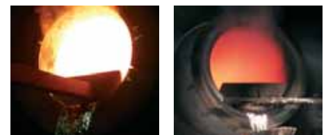
Casting from a rotary furnace (left) without salt-free addition (right with addition).
