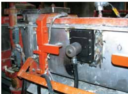
"Proxipro" Molten metal level sensor works on the induction principle
