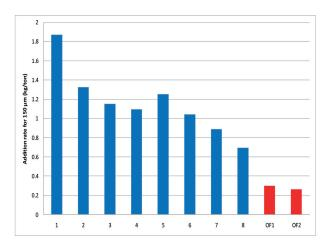
The chart shows that the amount of Optifine required to be added to achieve the required grain size of 150  $\mu m$  is reduced by 80% of standard addition.
