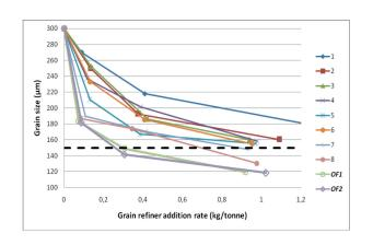
Grain refinement curves 1-8 show typical spread of efficiencies seen in coils provided by one supplier. Curves OF-1 and OF-2 for Optifine show high efficiency and consistent performance.
