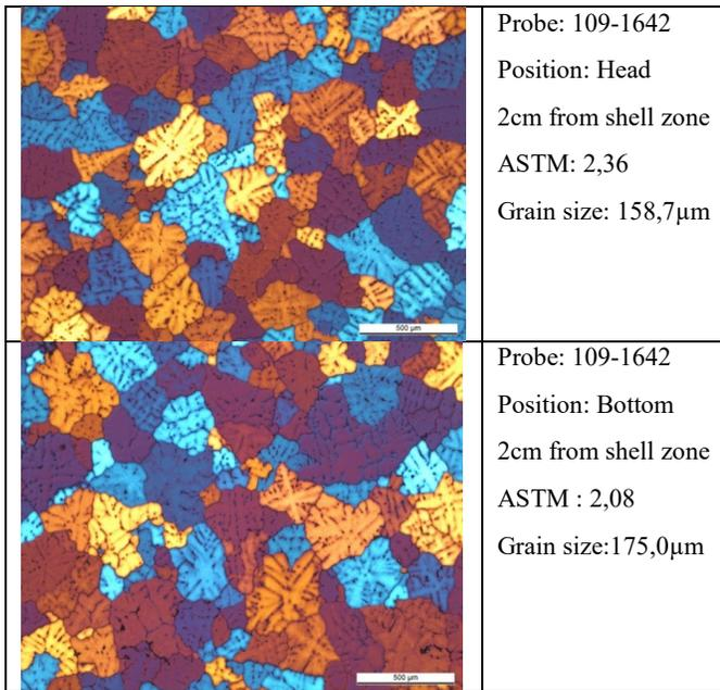
**Figure 3. Grain size measurement - Optifine grain refiner**
