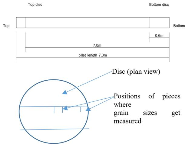
**Figure 2. Grain size measurement - standard grain refiner**
