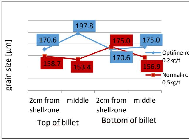
**Results of samples taken using Opticast sampler during production cast batch 109-1640 of 6060 billet (cast with 0.2kg/t Optifine)**
